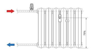
b. In the case of an even number of heating elements, when the radiator's mounting pin is located in the middle, the allocator (heat sink) can be moved one heating element toward the radiator's supply. The installation height should remain the same (75%):
