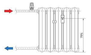
e. In the case of heaters with 20 or more elements 1 allocator should be installed. The rules of installation do not change and remain the same as in the cases described above:
