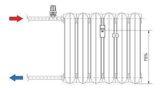
c. In the case of an odd number of heating elements and when it is not possible to install the allocator in the middle of the radiator's width, the allocator (heat sink) should be moved one heating element toward the radiator's supply. The installation height should remain the same (75%):
