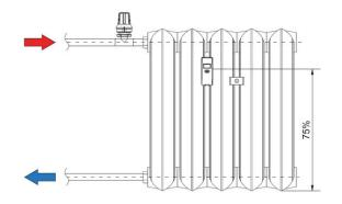
d. In the case of an odd number of heating elements and when it is not possible to install the allocator in the middle of the radiator's width, and when the mounting pin is located closer to the radiator's supply, the allocator (heating sink) is moved one heating element further. The installation height should remain the same (75%):
