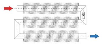
d. In the case of a 4-element radiator the allocator (heat sink) should be installed in the middle of the length of the first and third elements connection from the side of the supply. An example of such an installation is presented below.
